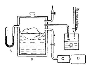
Scheme of the experiment to determine the oxygen absorbed by the animals. A) Water manometer; B) soda lime; C) pressure reducer; D) mixture poor in oxygen.
